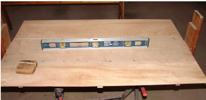
The jig's deck should be level prior to use.
